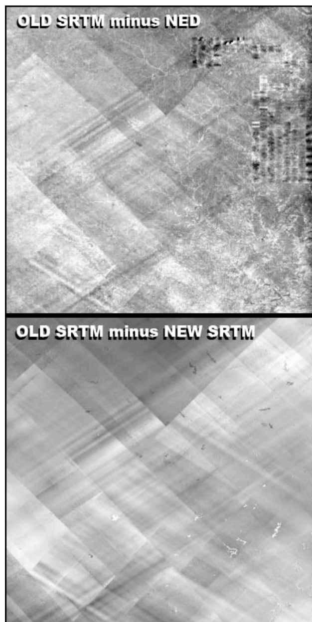
Figure 2. Old SRTM swath height errors evident versus both NED and the new SRTM, in which they have been reduced. Great Plains, USA, N35-40 W95-100.
