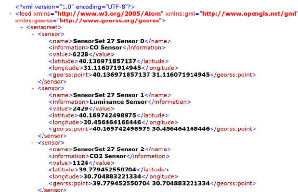
Figure 6. XML Representation of Sensors in Virtual Nodes
