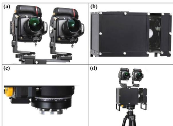
Figure 1. The Rotating Stereo Frame Camera System
