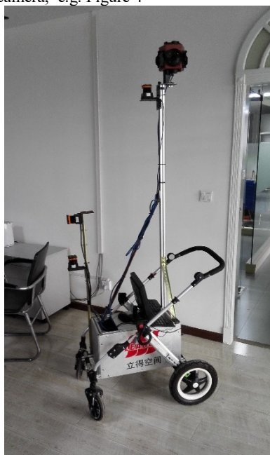
Figure 4. Indoor mobile measuring vehicle
