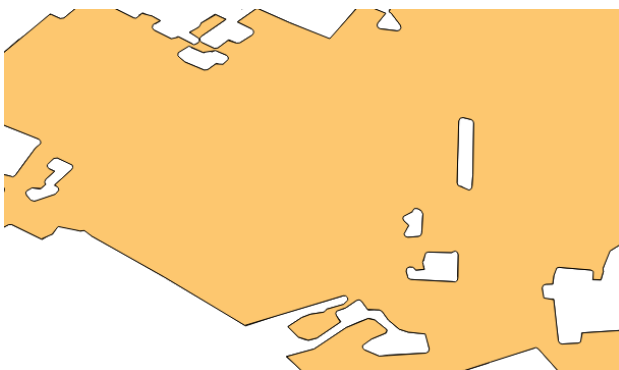
Figure 8. OSM built-up features after processing with a buffer distance x of 25m and a generalization distance of 5m.
