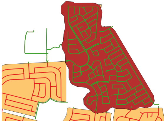
Figure 12. OSM residential roads (red: removed road segments after computing the difference with the resulting polygons of algorithm 1 [depicted in light orange]; green: remaining roads) and the resulting built-up areas (in brown) computed with an initial buffer distance y of 75m and a generalization distance of 5m (area of Darwin, Australia)
