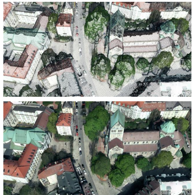
Figure 2. Texture mapped triangulated DSM raster showing vertices (top) and faces (bottom)
