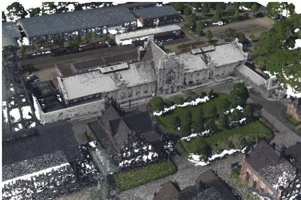
Figure 6. Coloured point cloud from software PhotoScan with overlaid TLS point cloud “Lohnhalle” in grey
