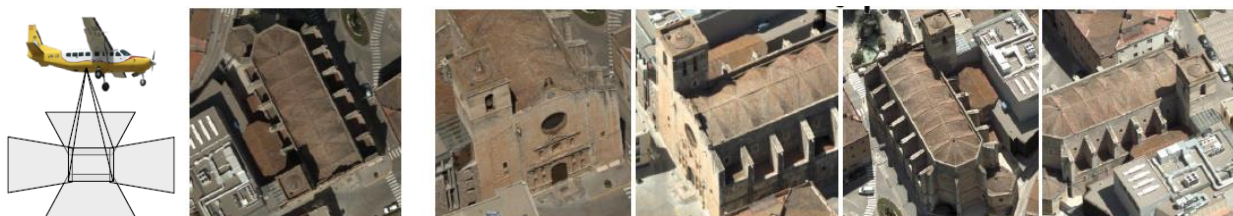
Figure 2: Maltese-cross camera acquisitions: a nadir view and the 4 cardinal views showing building footprints and facades.
