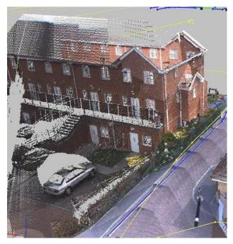
Figure 1. A coloured point cloud of a building in Eastleigh, captured using the MX8 mobile mapping system
