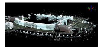
Figure 3. OS Explorer House point cloud captured using a Leica Pegasus backpack
