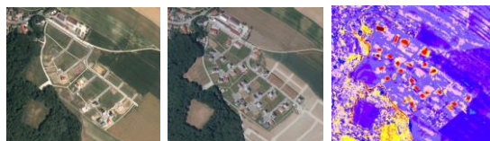
Figure 6. Differential DSM between LiDAR and Image Matching – new buildings are painted in red and areas under construction in violet
