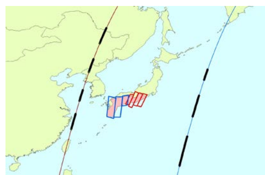
Figure 8. Illustration of FORMOSAT-2 Acquiring 7-Strips Images Data within 2 Hours by Using 2 Consecutive Orbits
