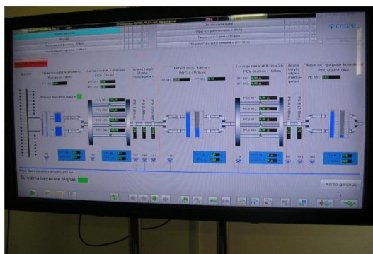
Figure 5. SCADA system main line
