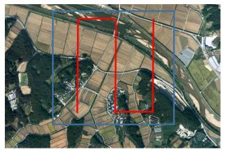
Figure 4. Test field and flight path with flight altitude of 200 m
