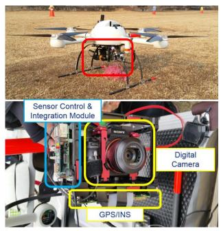
Figure 3. Hardware system of the UAV mapping system
