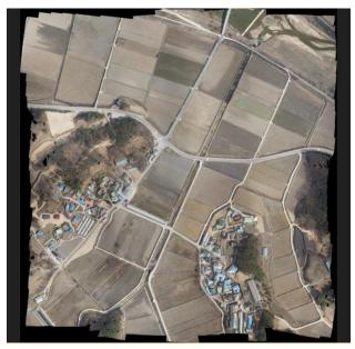
Figure 10. Orthoimage mosaic (flight altitude: 200 m)
