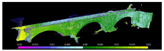
Figure 6. Comparison map [m] between the TLS point cloud and the photogrammetric model of the bridge.
