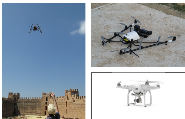
Figure 4. UAS used in this work. Left and upper right: AscTec Falcon 8. Lower right: Phantom DJ 3 Advanced.
