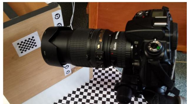
Figure 1. Camera with extension tube at the calibration field
