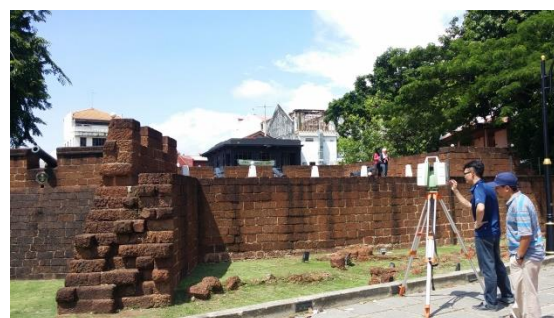
Figure 2. The scanning process from one of the scanning station
