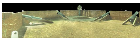
Figure 8. The coloured point cloud data of the top part of the monument
