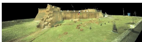
Figure 4. Visualizing of Bastion Middleburg monuments point cloud data from perspective view
