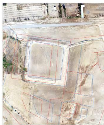
Figure 24 – RPAS orthophoto overlaid by FORMOSAT-2 orthorectified image, transformation parameters (rotation 0,085° and shift (33,310m in X axis and -7,067m in Y axis), FORMOSAT-2 in red and RPAS in blue
