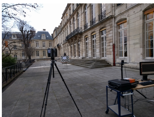
Figure 7: Experience on the evaluation of the accuracy of the distance measurement (outdoor)
