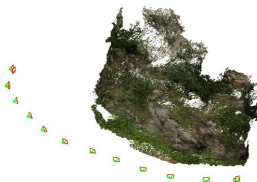
Figure 2. Example for a dense point cloud and the camera positions that were used for all cameras
