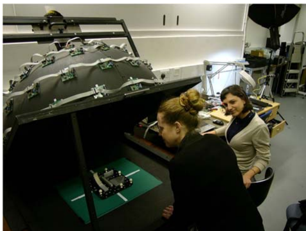
Figure 2. Positioning 3D test object on baseboard of dome.
