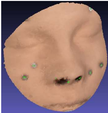
Figure 5: Phantom with screw heads defining reference locations. Green blob indicates automatic detection of the screw head.
