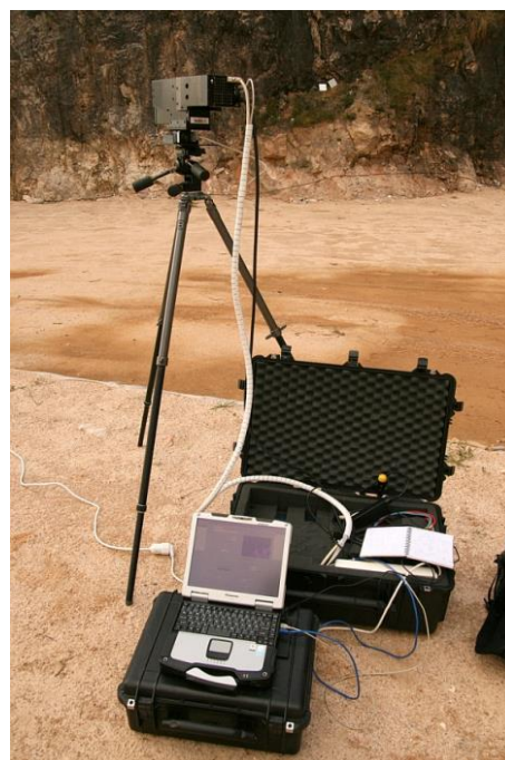
Figure 1. Tripod-based hyperspectral imaging for geological mapping of vertical cliff faces, showing HySpex SWIR-320m imager. The vertical scanning line of the sensor is moved on a rotation stage for image acquisition.
