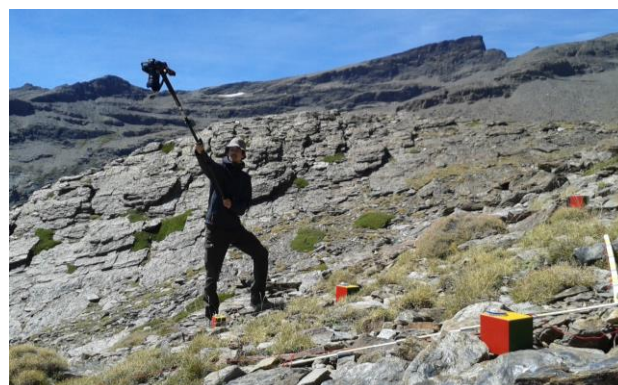
Figure 3. Image collection in the field with a camera attached to an extendable pole. In the foreground a target cube and wooden ruler
