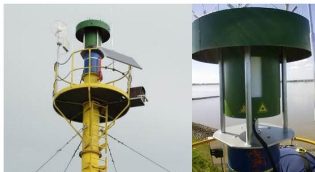
Figure 4. Complete system setup with case, solar panel and wind wheel (left), casing for the scanner on top of the platform (right)
