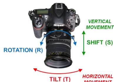
Figure 4. Movements of tilt-shift lens mounted on a DSLR camera with the image plane vertical and R=0^\circ .
