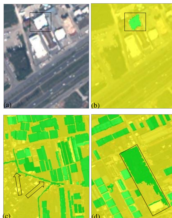
Figure 7. (a) White building. (b) Inaccurately classified white building. (c) Inaccurately classified road. (d) Inaccurately classified bare land.
