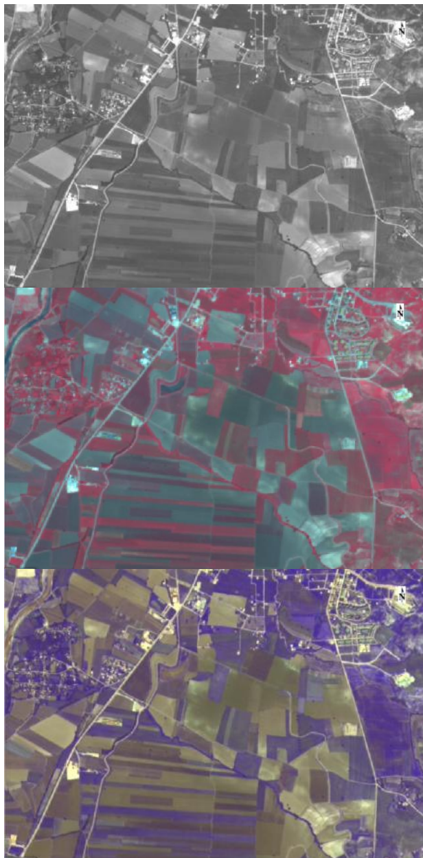
Figure 2. Panchromatic image, multispectral image and pan sharpened image.
