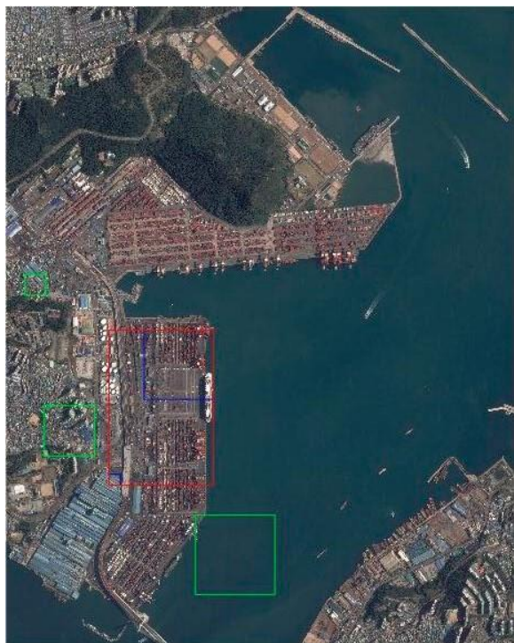
Figure 10. Detection on Busan Port in Republic of Korea by SIFT-based keypoint matching method
