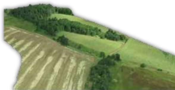
Figure 5. Digital surface model generated from UAV imagery by SfM algorithm
