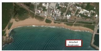
Figure 9. The simulation of wave crest after the placement of detached breakwater complexes
