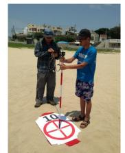
Figure 3. We used VRS system to survey the 18 GCPs
