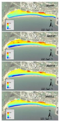
Figure 6. Multiple time series of beach DSMs
