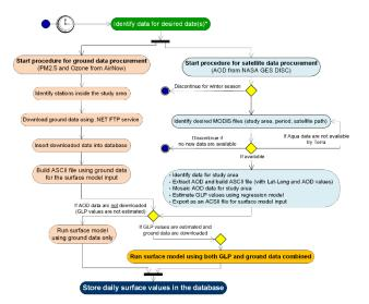
Figure 2. Process diagram for daily geospatial surface modelling for ground level PM2.5 (GPL) and ozone for GeoMedStat
