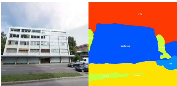
Figure 2. Input image and corresponding output from the FCN evaluation. The semantic class building is depicted in blue, sky in red, road in yellow, plant in green and car in bright blue, respectively.
