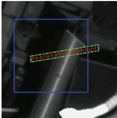
Figure 3. The IMBLS search window (green) and a classical, rectangularly-shaped search window (blue) around the candidate homologue point. (The red dots are the candidates corresponding to every h_k .)
