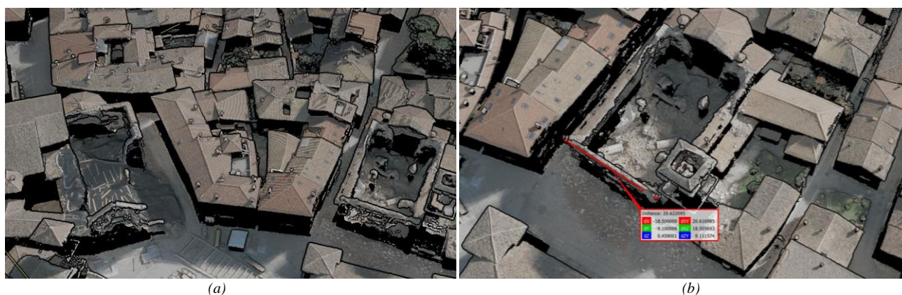
Figure 8. Shaded 3D point cloud of Norcia with RGB information
