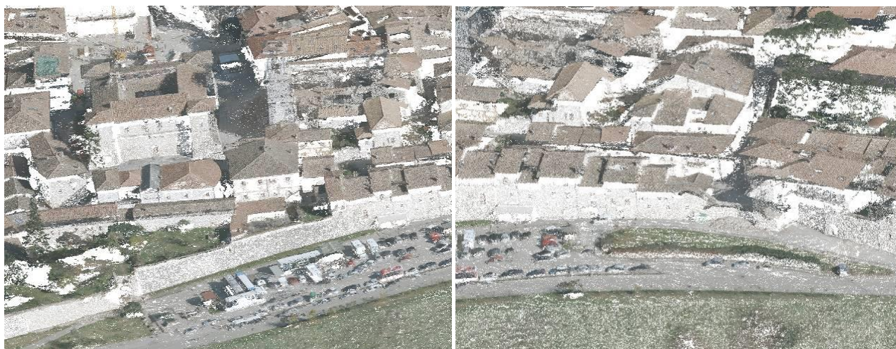
Figure 7. 3D point cloud of Norcia with RGB information.
