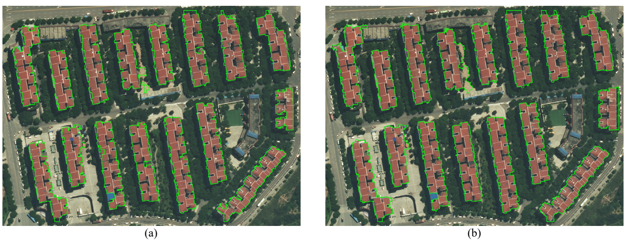
Figure 3: For image 5, (a) Result of building contours extraction using ORB+BBOF; (b) Result of building contours extraction using SURF+BOF.
