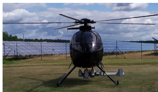
Figure 4. Phase One iXU-RS 1000 digital camera and RIEGL LMS-Q680i laser scanner on the suspension of Hughes MD 500 helicopter
