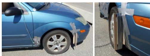
Figure 1. Ultrasonic sensor installation on the front right wheel of a Ford Focus Car.
