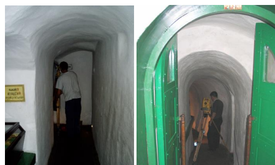
Fig. 4. Scanning stations georeferencing by free station method
