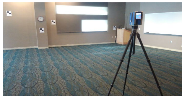
Figure 2. Test field scanning by FARO Scanner
