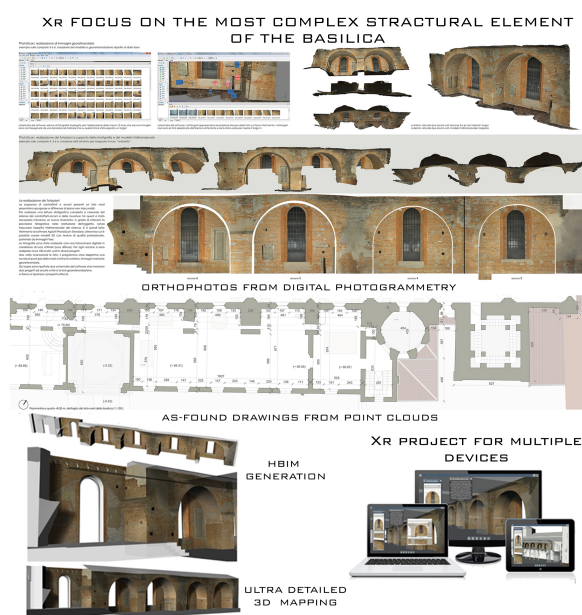
Figure 12. The Xr contents related to the focus of the double-waved curve wall: different data sources have been used for a detailed 3D mapping in Unreal Engine 4.
