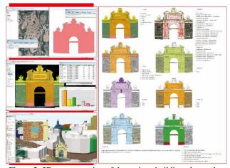
Figure 2. 3D reconstruction of the various building phases that have affected Porta Valbona
