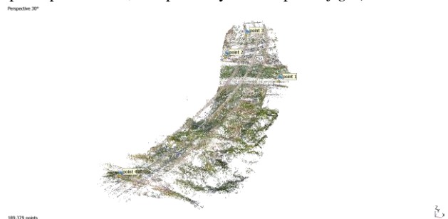
Figure 7. Annunziata Viaduct sparse point cloud
