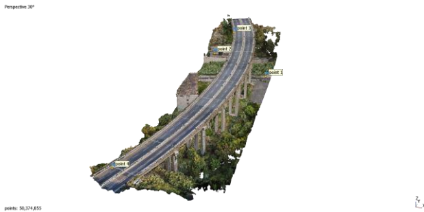
Figure 8. Annunziata Viaduct dense point cloud
