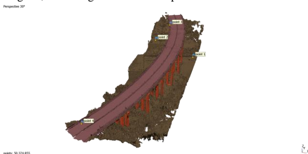
Figure 10. Annunziata Viaduct classified point cloud with deck (pink) and pillar (red)
