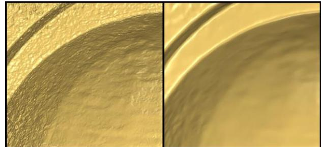
Figure 7. On the left: mesh (automatically generated) with topological errors. On the right: final mesh after editing operations.
