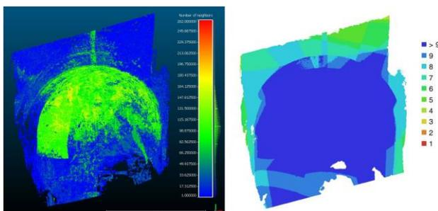
Figure 6. On the left, point cloud density analysis displayed on the point cloud. On the right, image overlap scheme.
