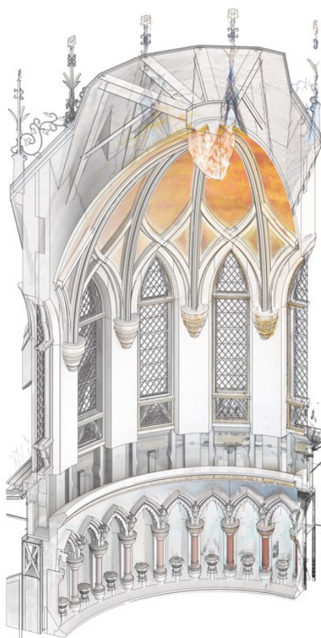
Figure 7: Sectional View of Library of Parliament BIM Lantern with coloured point cloud overlay.
