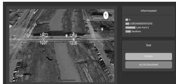
Figure 10. user interface to handle geophone sensors.
