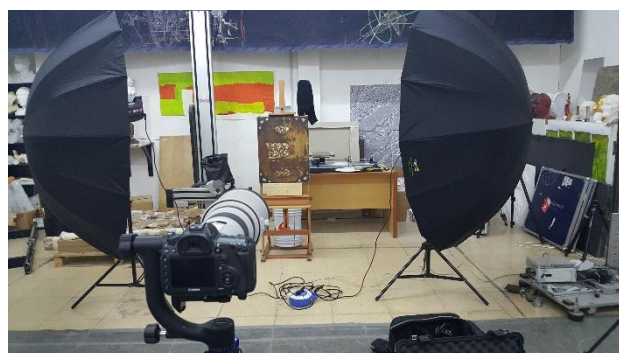
Figure 5. Colour photography capture setup for the unnamed 17 th -century painting
