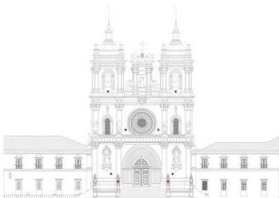
Figure 14. Location of the five control points for the photogrammetric survey of the facade of the monastery of Alcobaça (Coelho, Genin, 2016).
