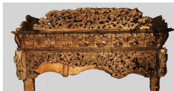
Fig. 3a Point cloud from automatic SfM procedure without manually introduced tie points
