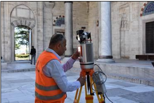
Figure 6. Riegl VZ-400 laser scanner at Suleymaniye Complex
