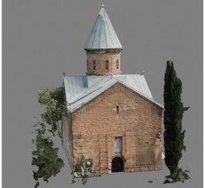
Figure 11. Textured and meshed 3D model from PhotoScan (Alignment "medium", Dense cloud "high", Mesh "arbitrary, high", Texture "adaptive orthophoto, mosaic")
